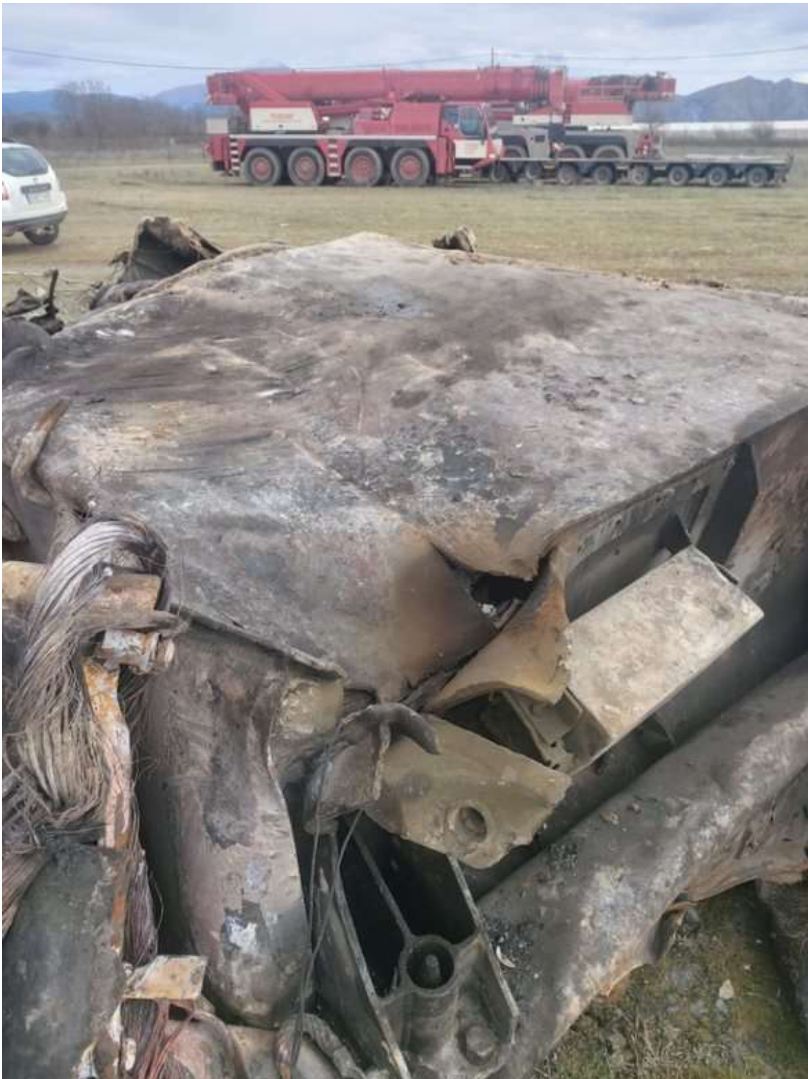
Figure 16: Transformer 120023 with explosion hole - file: 230307_123509.jpg
