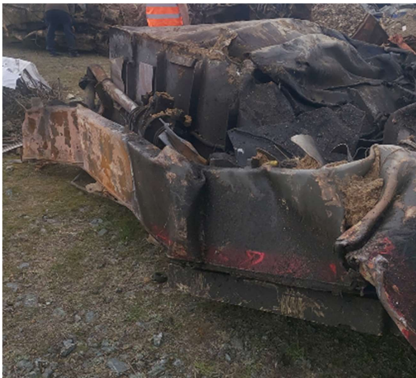
Figure 22: Transformer opposite site explosion & fire hole (extract file : 20230307_124.106.jpg)
