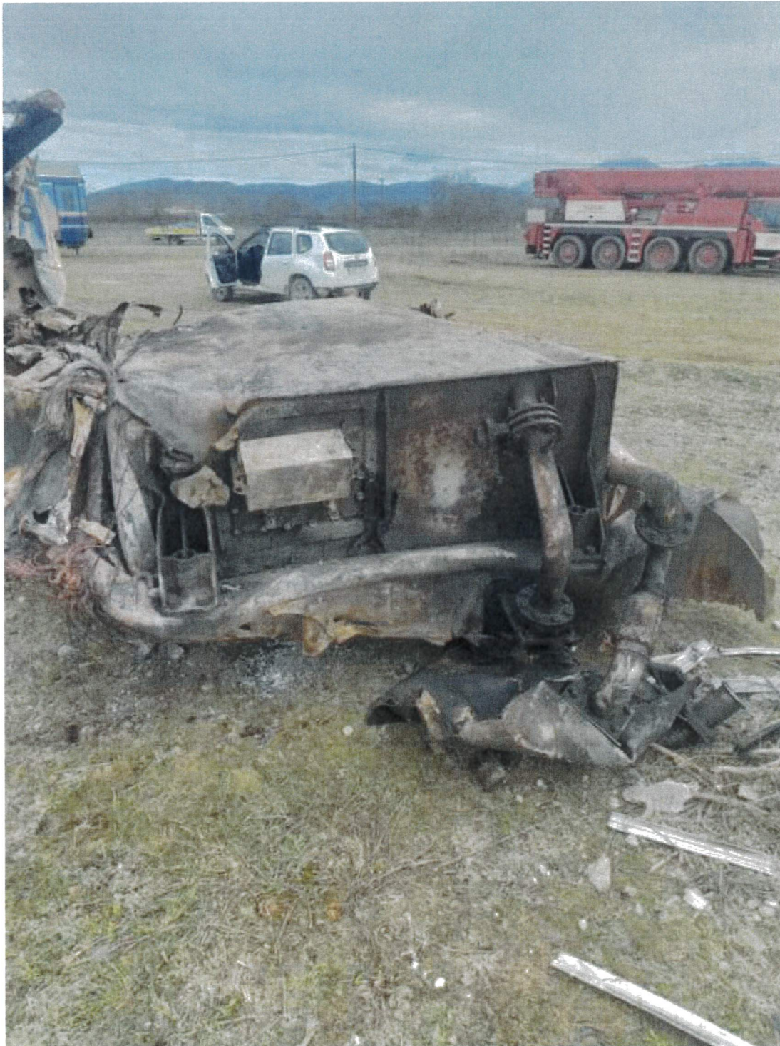
Figure 19: transformer from same view as drawing (here upside down in debris)
