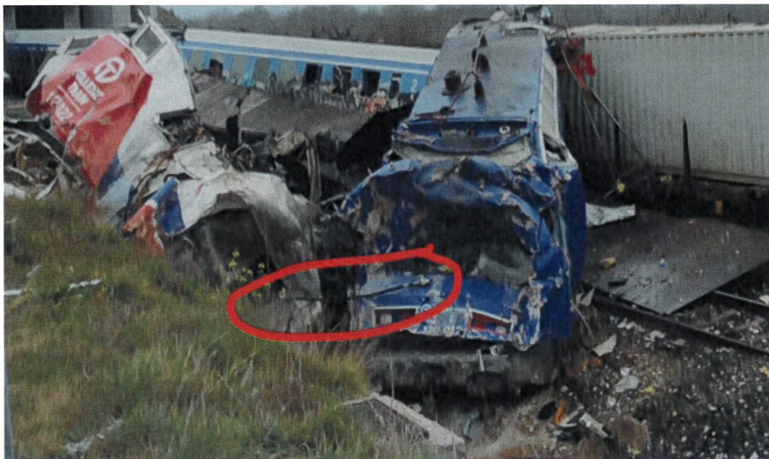
Figure 13: Freight locomotives - Still electrical connected (UIC-plugs) (20230301-071311.jpg)
