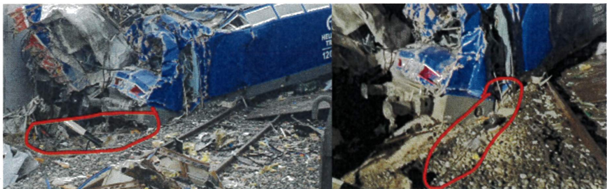
Figure 12: Catenary line under freight locomotive (20230301-105223.jpg & 20230301-034238.jpg)
