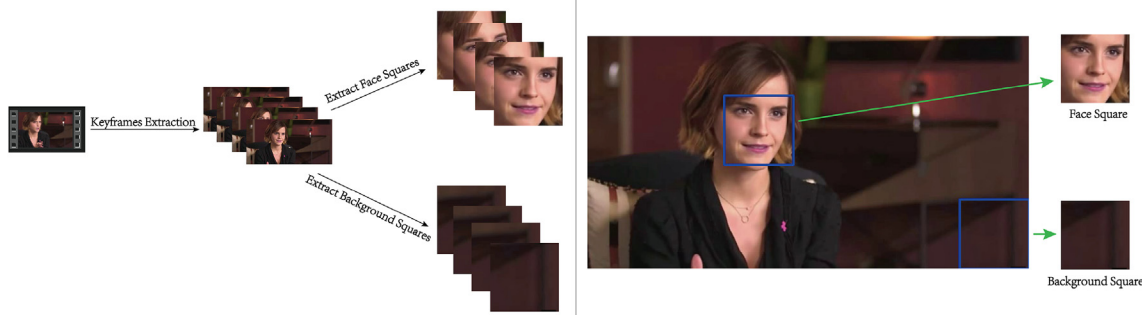
Fig. 2. Keyframes are extracted from the Deepfake video, then the face and background squares are cropped from each keyframe. The face square in a keyframe is detected and cropped using the dlib library, and a background square with the same size and having the furthest Euclidean distance from the detected face within the image frame is found and cropped.
