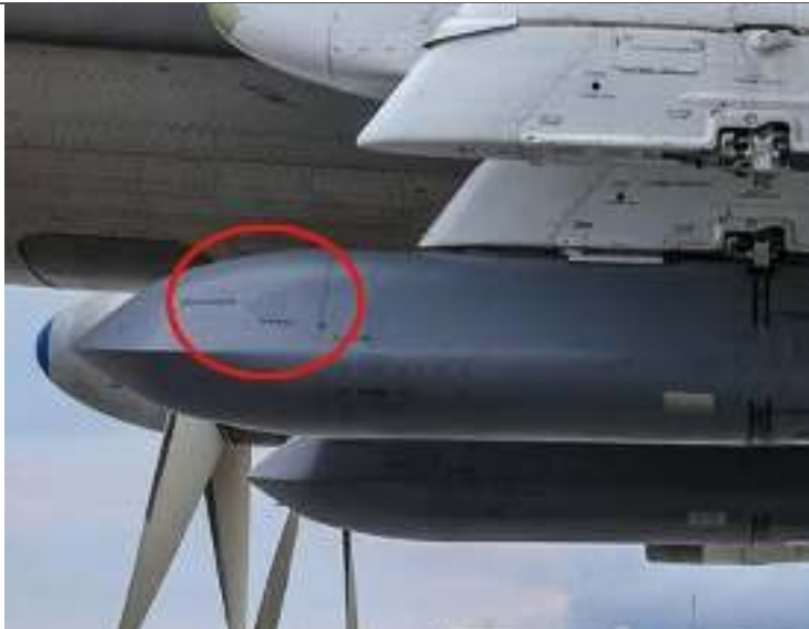
Ventilation holes and serial number on the front of the rocket
