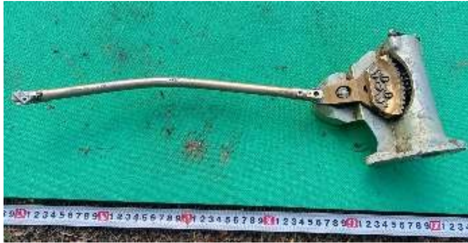
Figure 50 - 3M-14 rudder linkage and mechanical transmission
