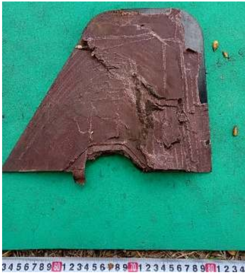
Figure 47- Damaged composite rudder fins on the 3M-14 shank
