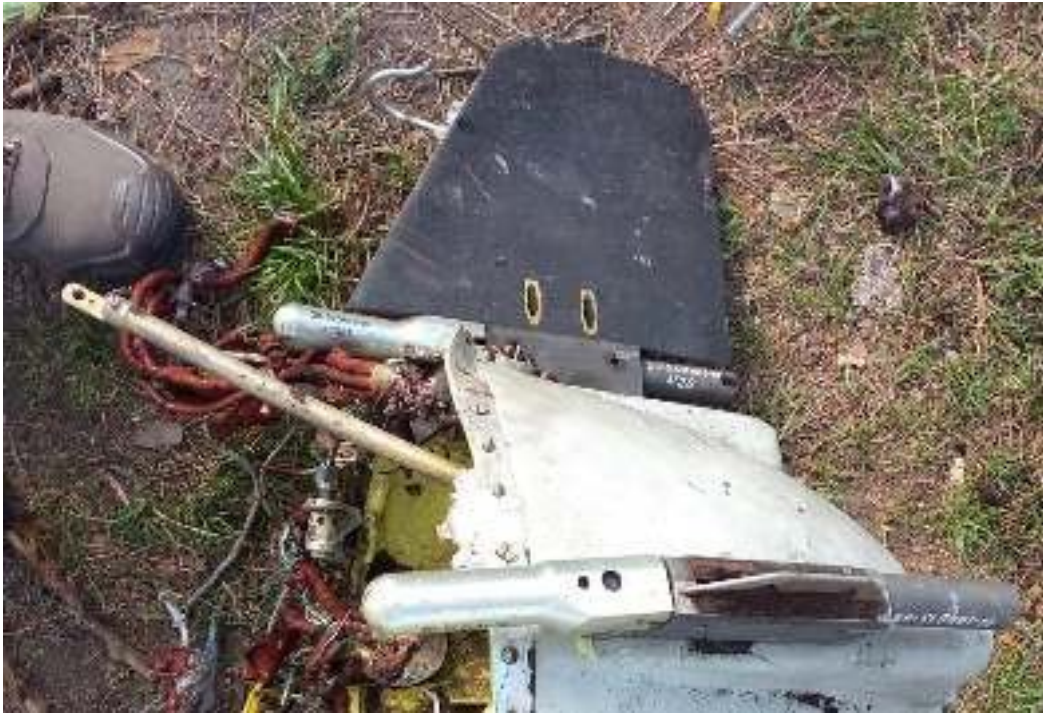
Figure 46 - Composite rudder fins on the 3M-14 shank
