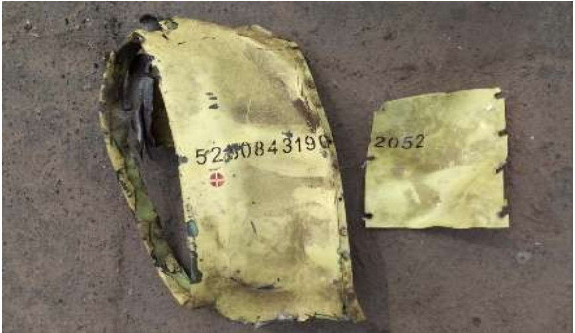
Figure 22 - Engine cowling with serial number "52808431902052"
