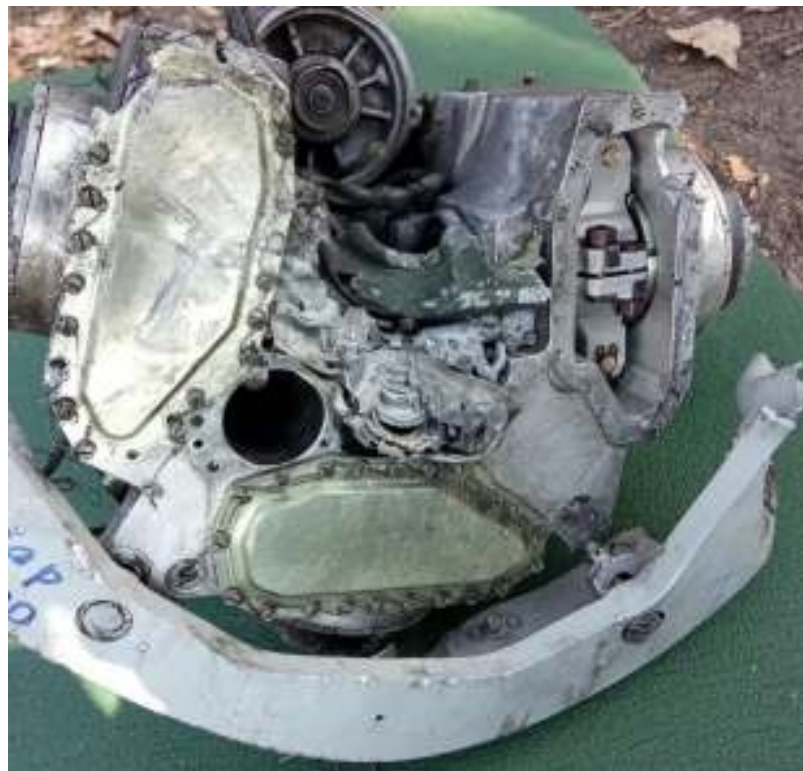
Figure 28 - K-005 rudder actuator unit
