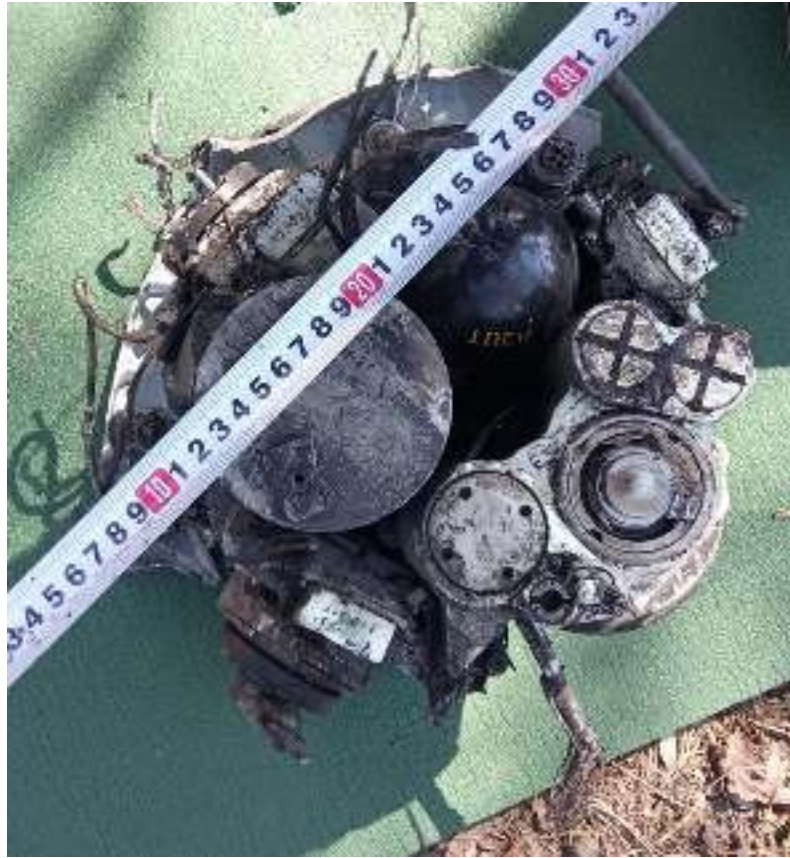
Figure 27 - K-005 rudder actuator unit
