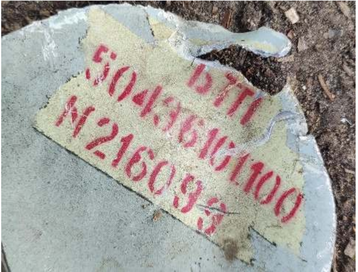
Figure 31 - Example of "504E" marking - a fragment of the fuel supply system
