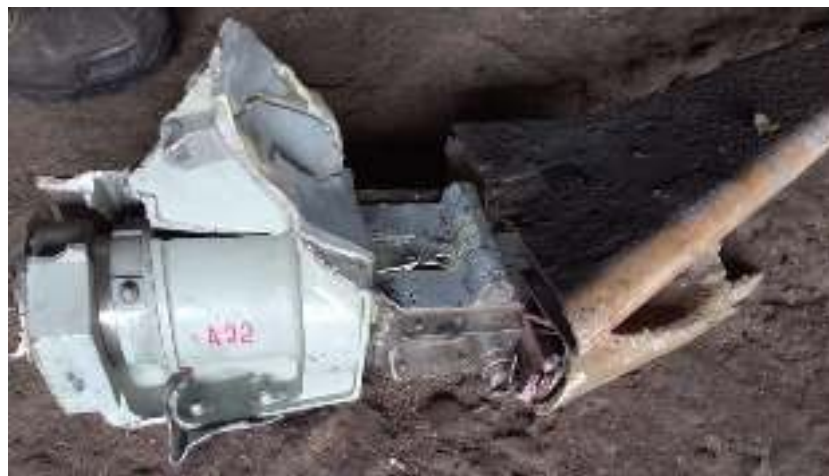
Figure 34 - Fastening lock, swivel mechanism labeled "A22" and a fragment of the left horizontal plane of the rudder
