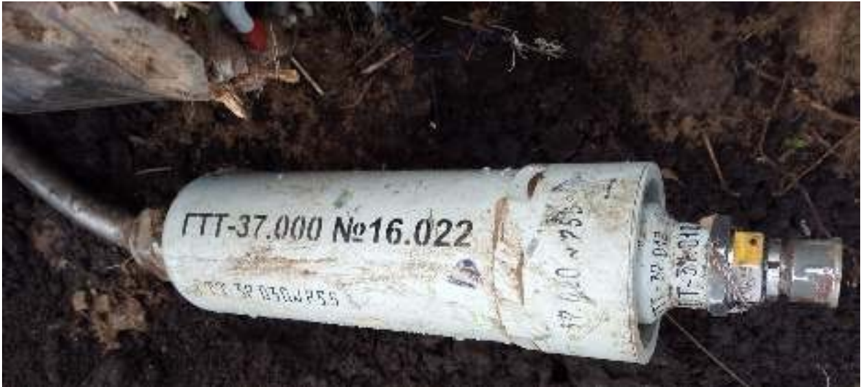
Figure 61- Remote unit marked "GTT" - a distinctive feature of the TRDD-50B engine that distinguishes it from the TRDD-50A (X-101) and "Product 64M" (X-35U)
