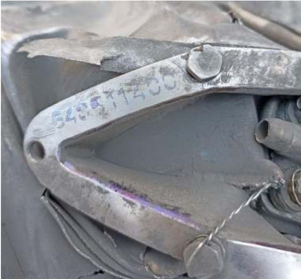
Figure 9 - Example of marking on the motor "Product 64M"
