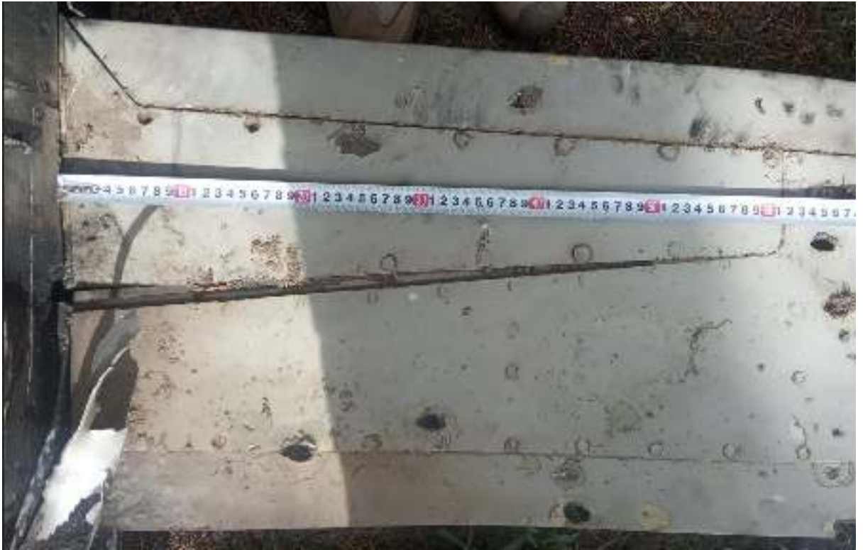
Figure 57 - The Caliber and Iskander wing spar is 61 cm long, as opposed to 170 cm for the X-101
