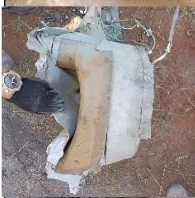
Figure 54 - Material of the insulating lining of the air inlet edge
