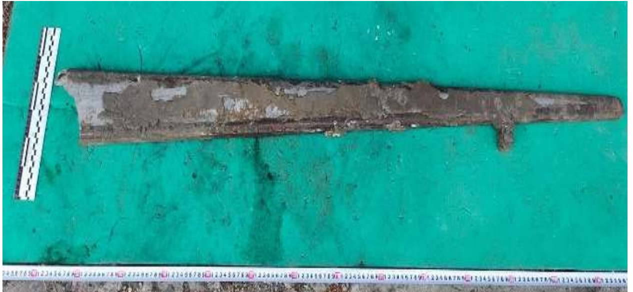
Figure 25 - Support spar of the X-101 cruise missile
