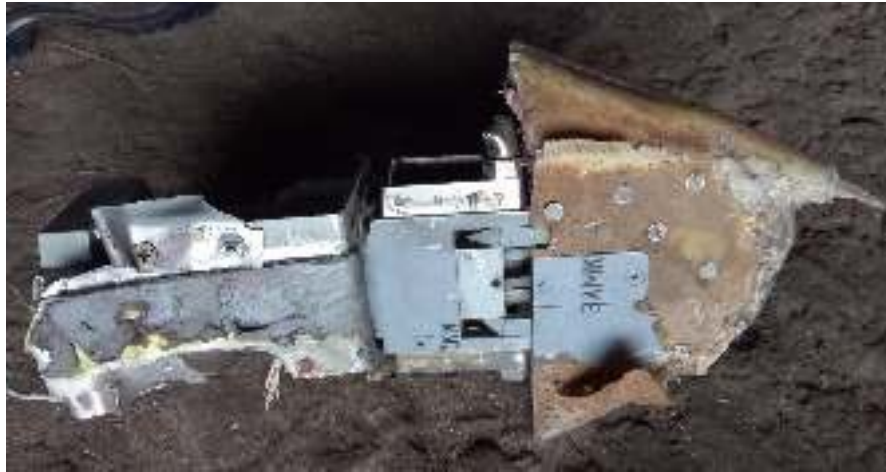
Figure 33 - Rudder tail fin attachment lock
