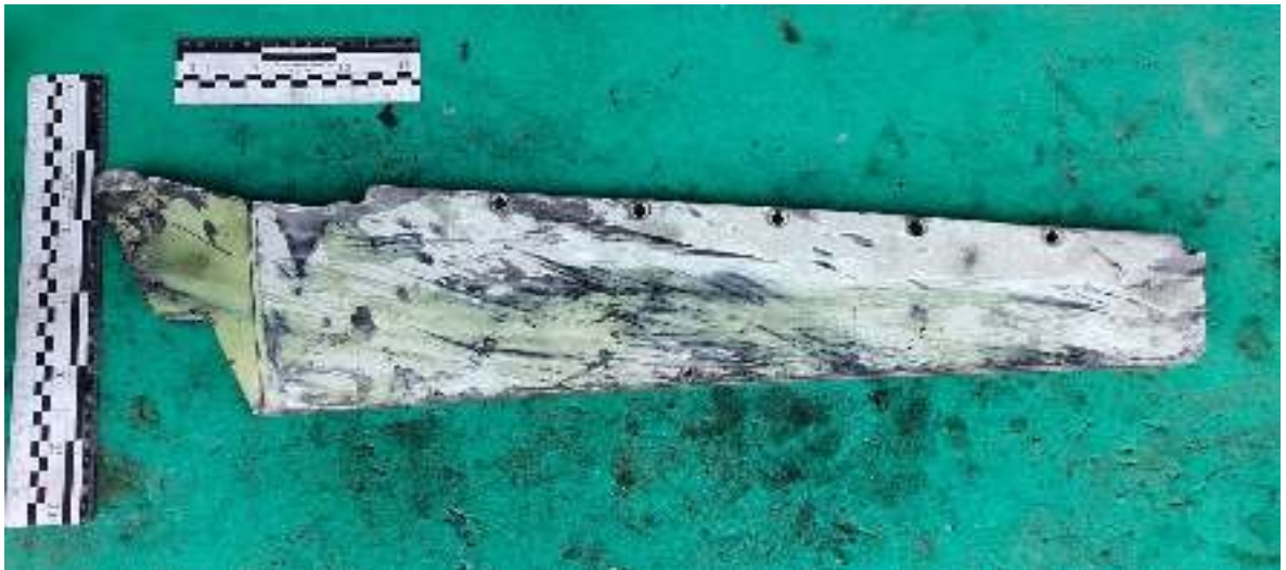
Figure 23 - Support spar of the Kalibr cruise missile
