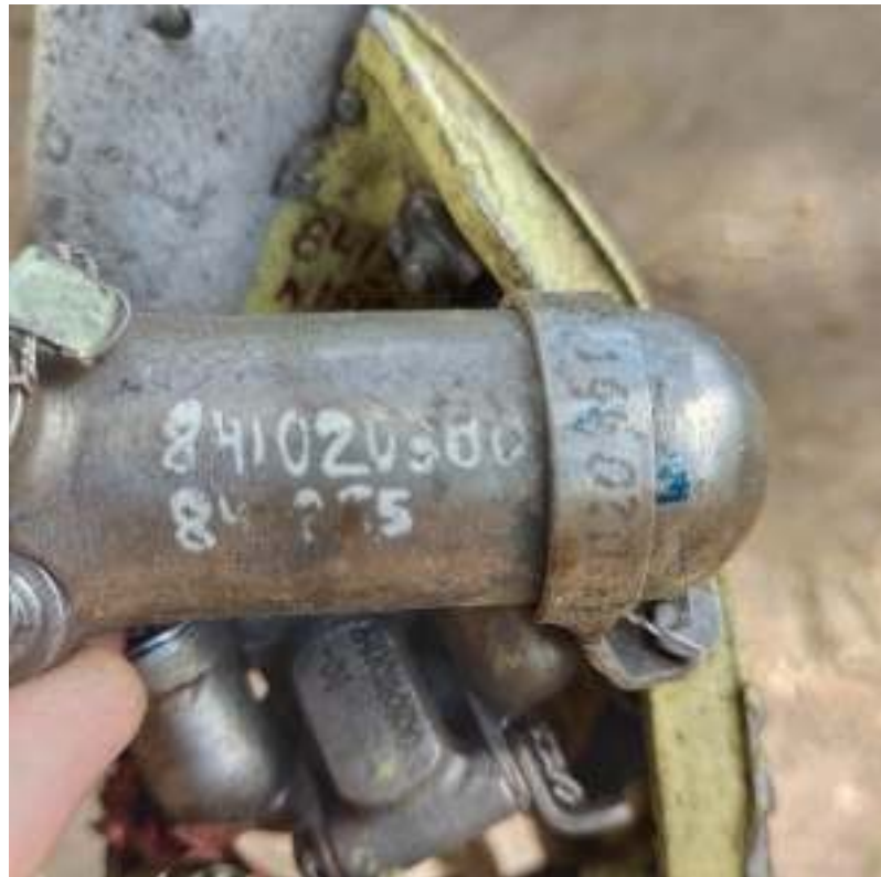
Figure 32 - Example of labeling with the digits "84" at the beginning of the number
