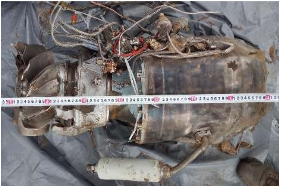
Figure 60 - Exterior view of the TRDD-50B engine
