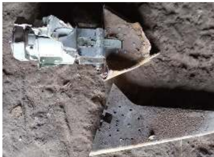
Figure 35 - Fastening lock, swivel mechanism labeled "A22" and a fragment of the left horizontal plane of the rudder
