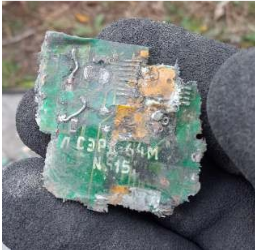
Figure 13 - Fragment of the board labeled "SERD-64M" (the name of the engine control system "Product 64M")
