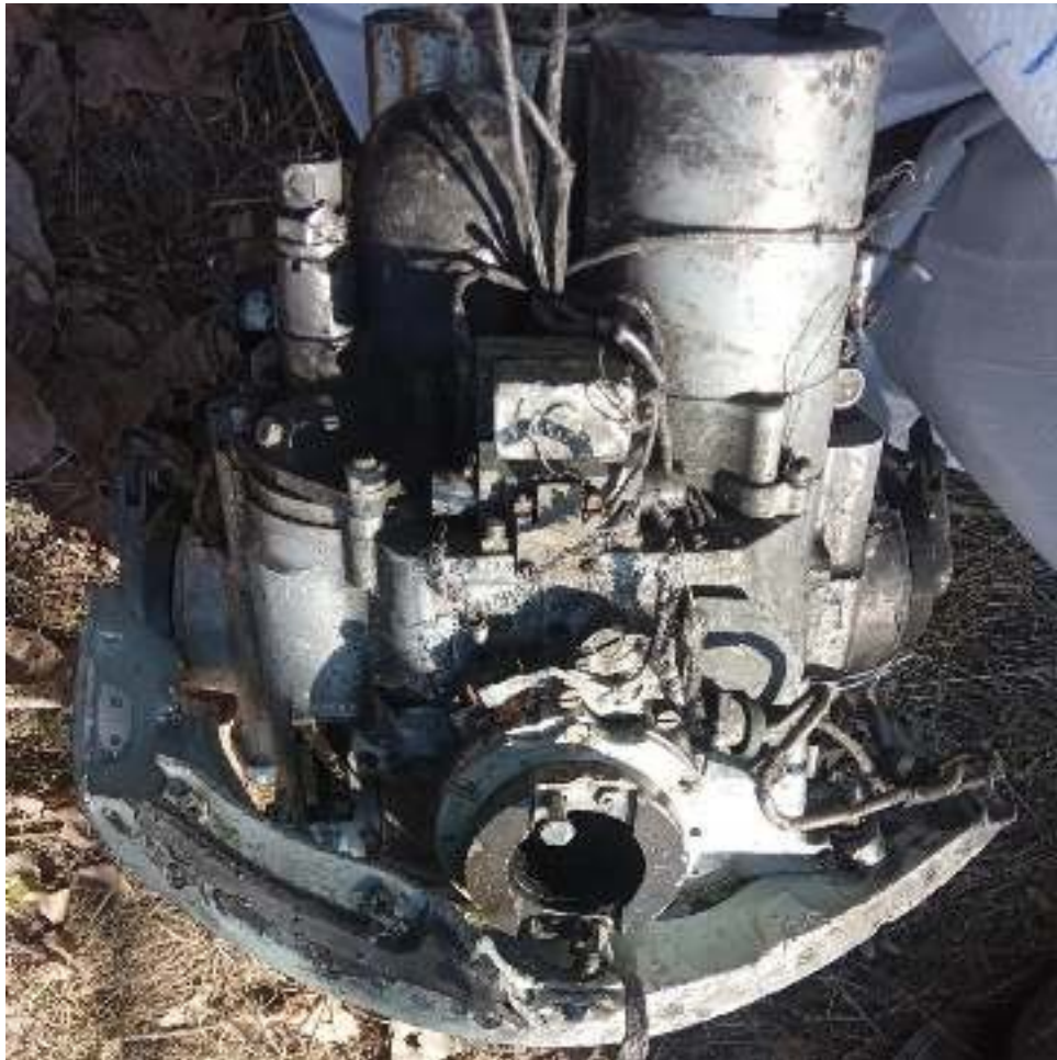
Figure 26 - K-005 rudder actuator unit
