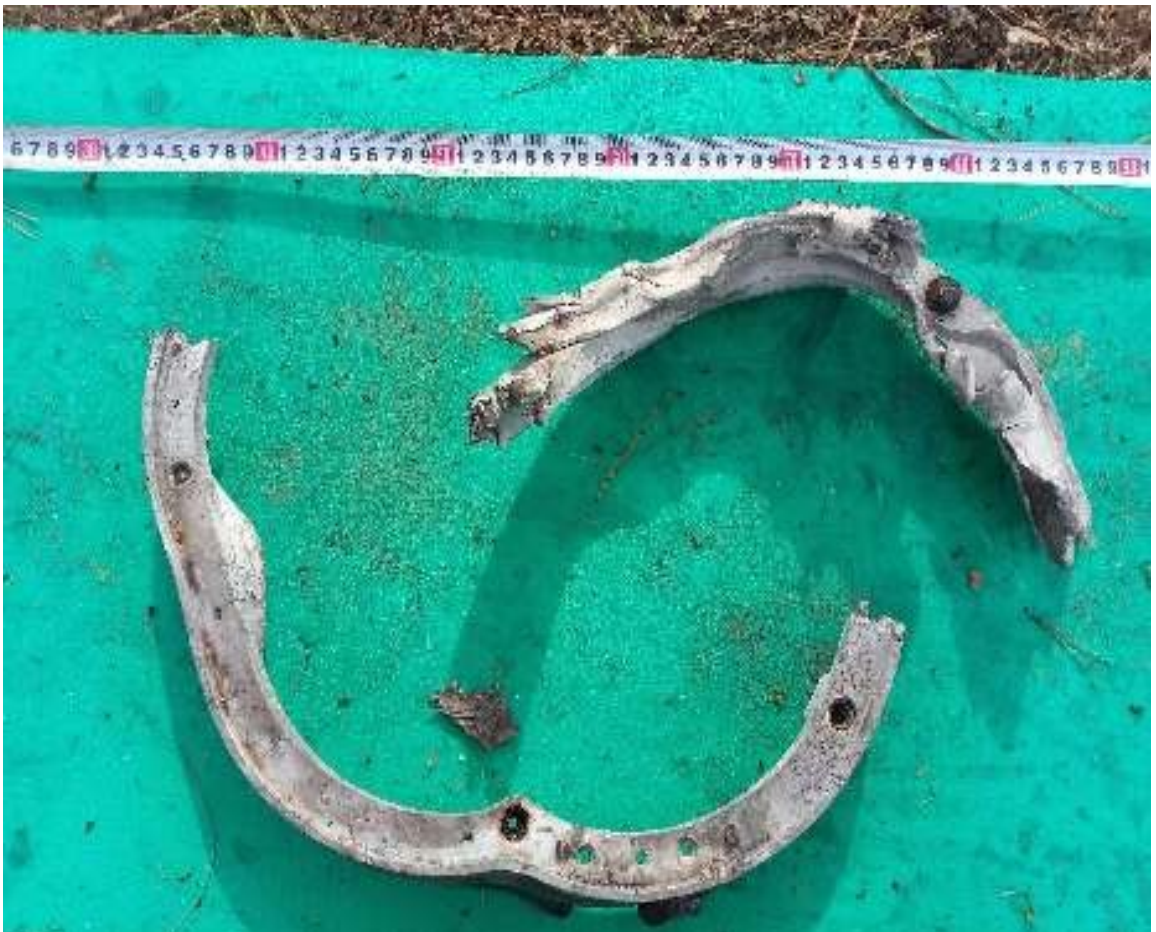
Figure 6 - Support frames with an octagonal shape
