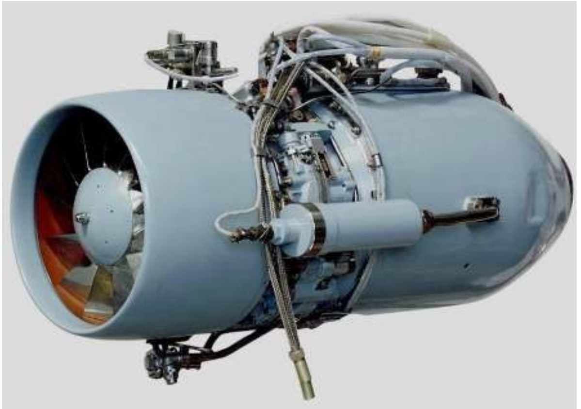
Figure 59 - Exhibition model of the TRDD-50B engine ("Product 37-01")
