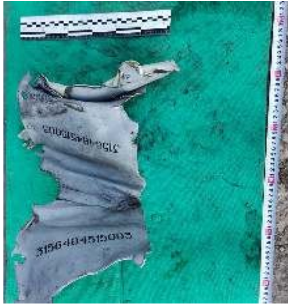
Figure 20 - Serial number of the X-101 missile "3156484515003" The decoding of the serial number is shown in Table 5.
