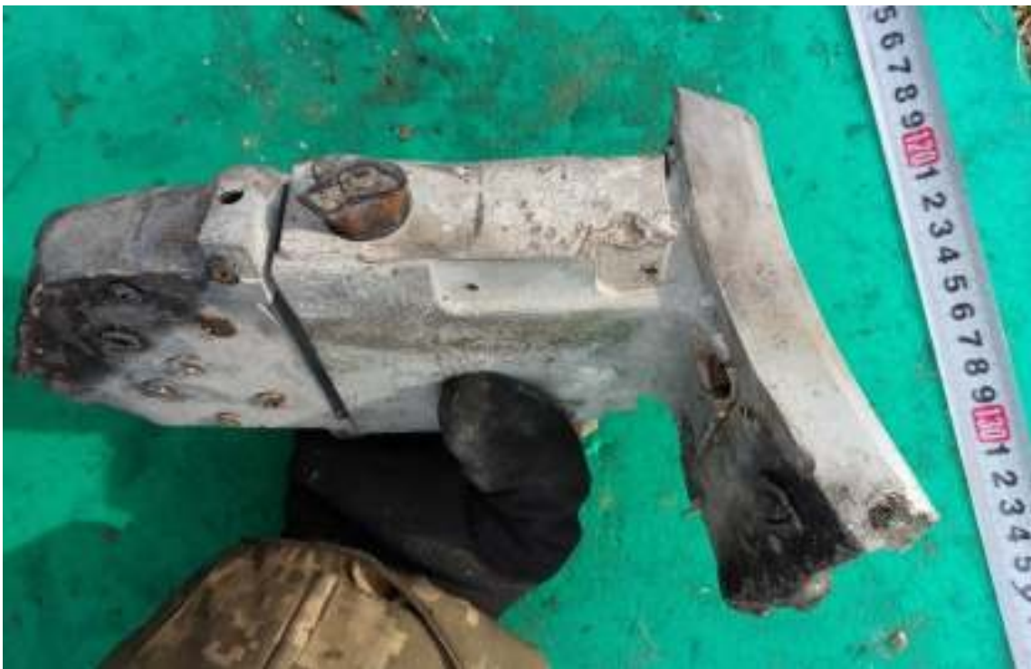
Figure 8 - Mounting of the missile's front fin
