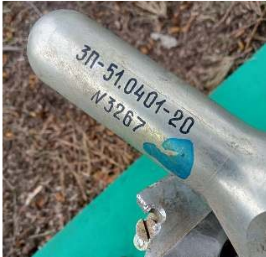
Figure 48 - Typical 3M-14 rudder markings
