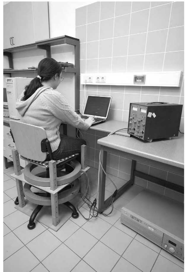
Fig. 1. The experimental situation. The Helmholtz-coils below the chair were only virtually connected to the power supply hence no electromagnetic field had been generated at all.
