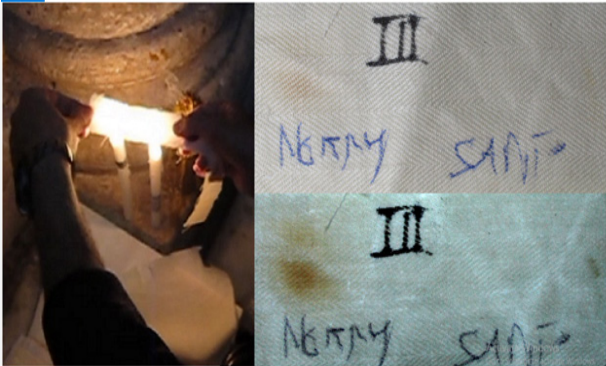
Figure 9: Third experiment of bleached TS-like linen fabric exposed to fires for about 4s. The CF produces a more evident singeing than the HF, better visible in UV on the bottom. On the Left, set-up of this experiment.
