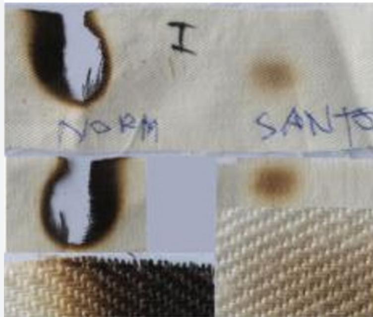
Figure 7: First experiment of bleached TS-like linen fabric exposed to fires for about 30 s. “The CF (on the left) burns the linen, while the HF (on the right) only sines it.”
