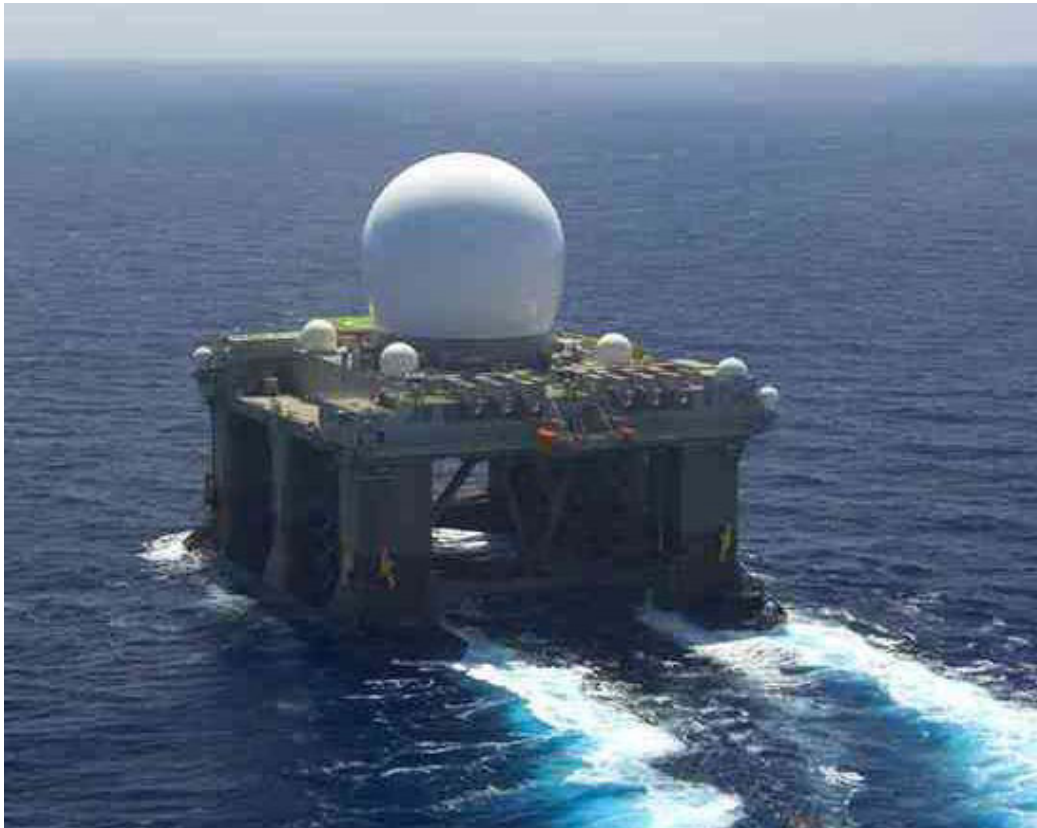
The Sea-Based X-Band Radar (SBX-1) maneuvers in the Gulf of Mexico during initial at-sea testing in July, 2005.
