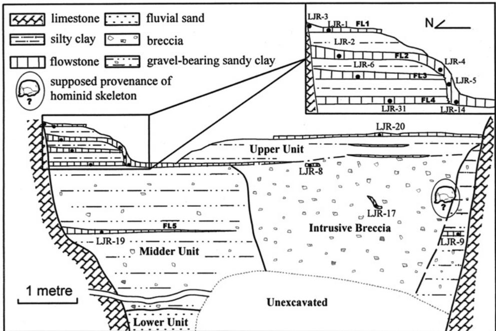
Figure 3. Sketch showing three depositional units and Refilling Breccia on the extant cross-section, which corresponds to the line AB in Figure 1. Samples for dating were collected from the five flowstone layers and other speleothem formations. Here the encircled skull denotes the probable provenience of the hominid skeleton.
